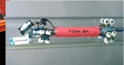
"In pipe" inspection microrobot (weight: 16g) (Toshiba, Japan)
